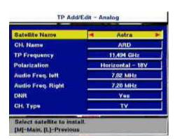
Now press the button to select the required satellite and, using the number buttons, enter the channel name (see section "Notes on operation").
